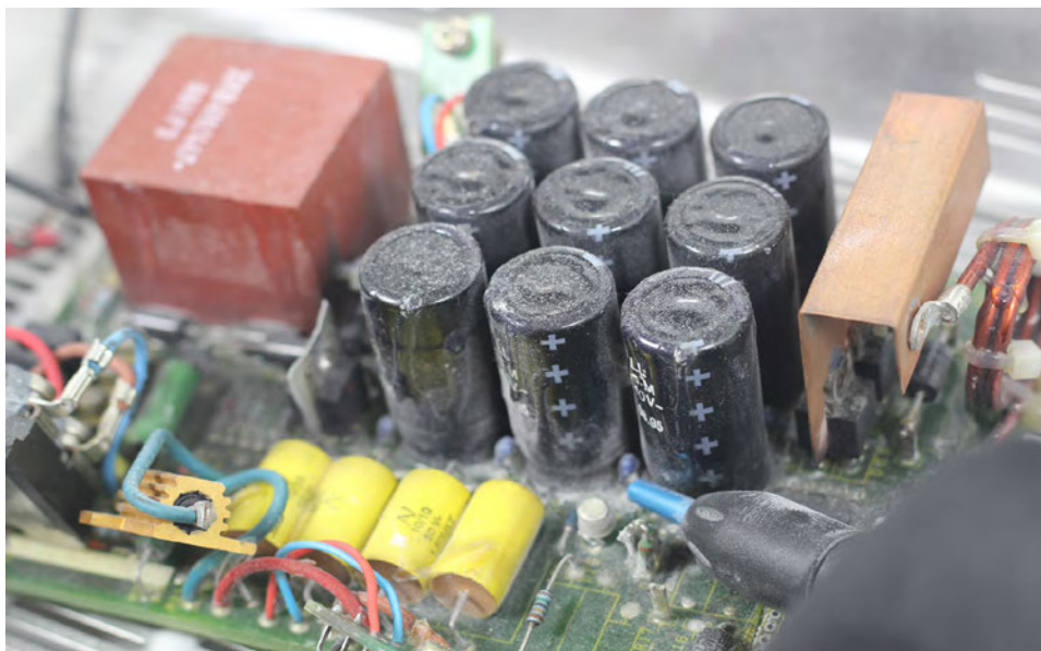
Figure 3: Coating removal using micro blasting technique.
