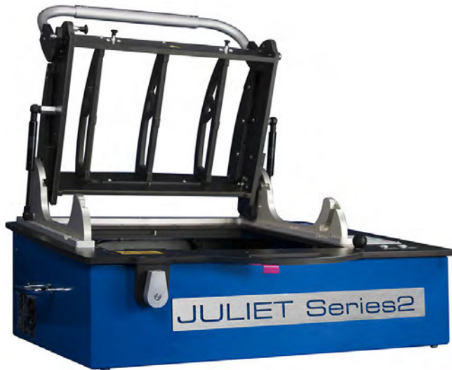
Figure 10: Combination tester for the synchronized use of external tools and all embedded system access technologies on one platform.
